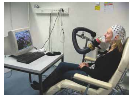
Proband attached to olfactometer ©Institute of Experimental Psychology, Department of Biological and Social Psychology
